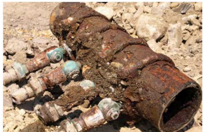
Corroded water main with lead fittings. Photo by Mike Thomas via Flickr, CC BY NC ND 2.0
